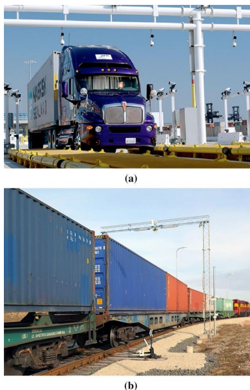
Figure 5. OCR recognition a) Trucks and b) trains
